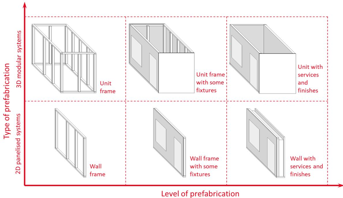
Figure 1: Type and level of prefabrication
