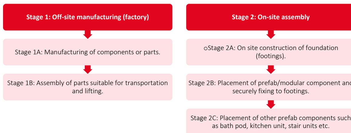
Figure 2: Two key stages of construction for prefab and modular housing
