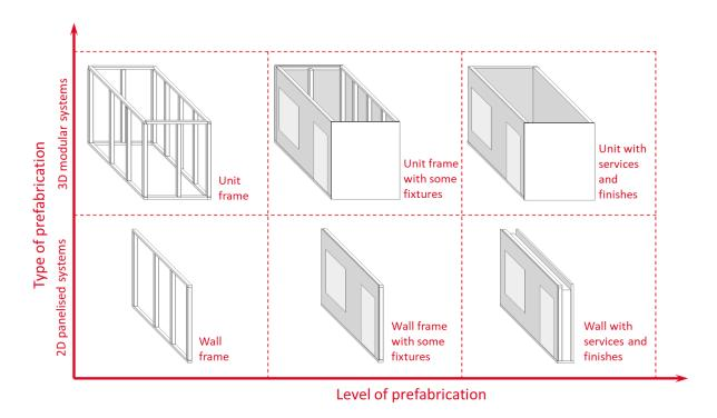
Figure 1: Type and level of prefabrication
