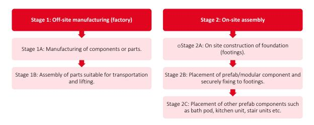
Figure 2: Two key stages of construction for prefab and modular housing
